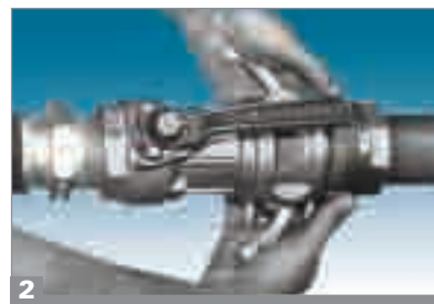
2 Cam Arms Lock Coupler and Adaptor Together
